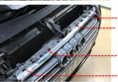
7 Carefully pull the bumper free from the corner at each side. Do not attempt to remove the bumper at this stage, only disengage the sides of the bumper from the chassis clips
