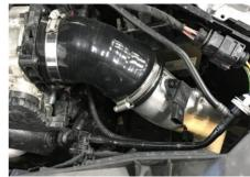
Refit the MAP sensor using the M6x10mm socket head bolt provided. Reconnect the multiplug and push in the red tab to secure, note that the wiring will need to be run around the rear of the pipe now.
