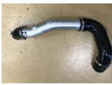
Fit the supplied new hose clamp over the intake manifold end of the Revo throttle pipe and fit to the intake manifold. Do not tighten yet
