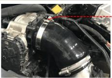
16 Fit the supplied new hose clamp over the intercooler end of the Revo throttle pipe and fit to the intercooler. Do not tighten yet
